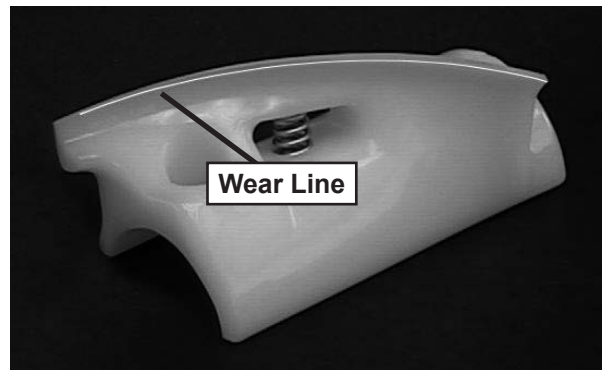
Figure 3-3 Auger Flight Wear
