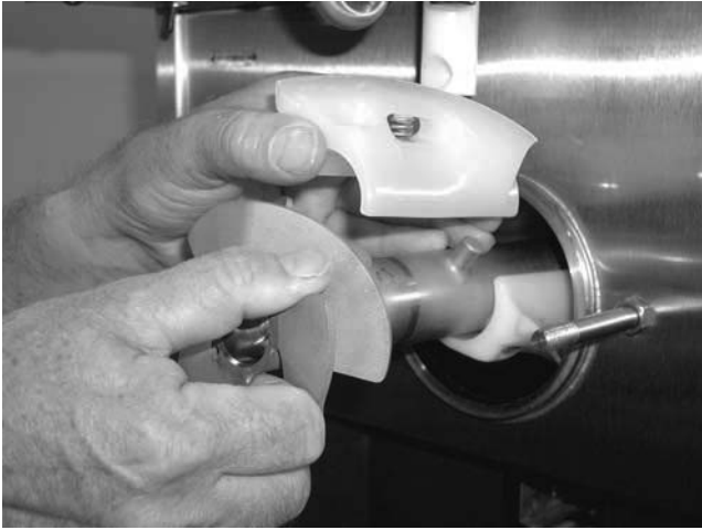
Figure 22. Auger Shaft Removal
