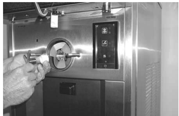
Figure 21. Removing Auger Support
