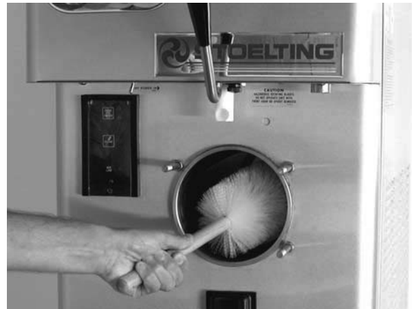
Figure 17. Cleaning Freezer Barrel
