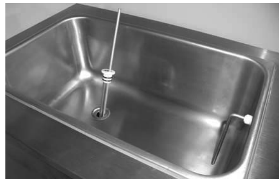
Figure 12. Removing Mix Inlet Regulator (Shown with no mix in hopper)
