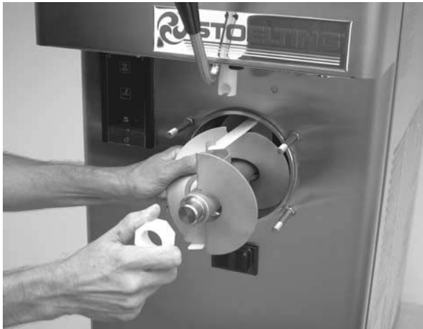
Figure 15. Auger Shaft Removal
