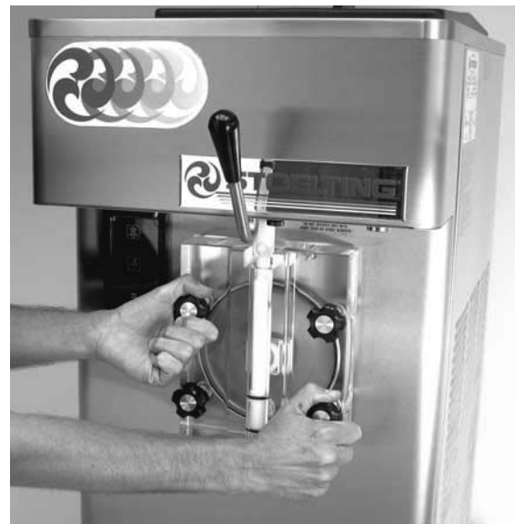
Figure 14. Removing Front Door
