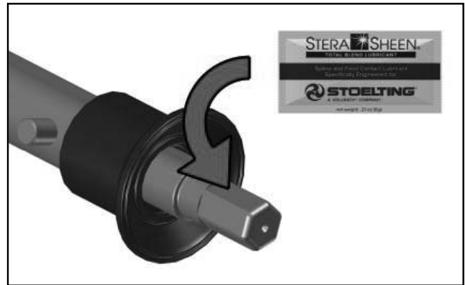
Figure 3-6 Lubricate Hex End of Auger
