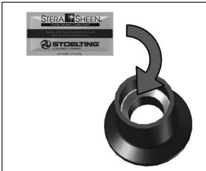
Figure 3-5 Lubricate Rear Seal
