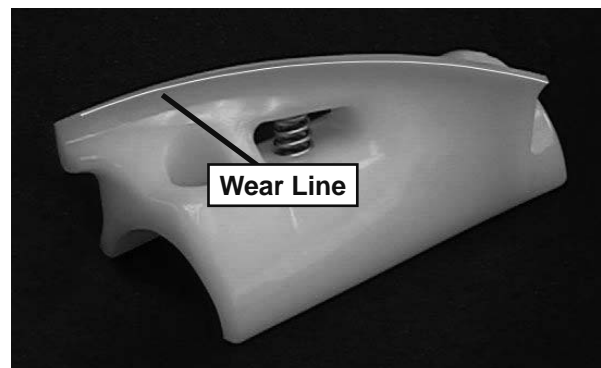
Figure 3-3 Auger Flight Wear
