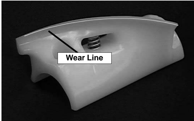
Figure 3-3 Auger Flight Wear
