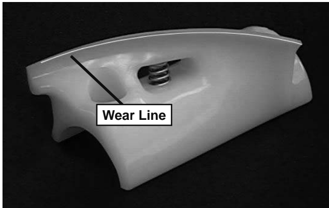
Figure 3-3 Auger Flight Wear
