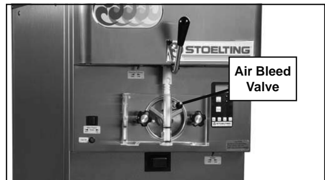
Figure 3-8 Air Bleed Valve
