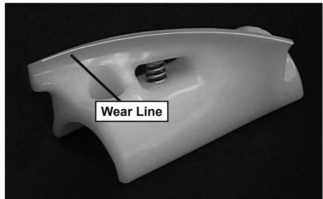
Figure 3-3 Auger Flight Wear
