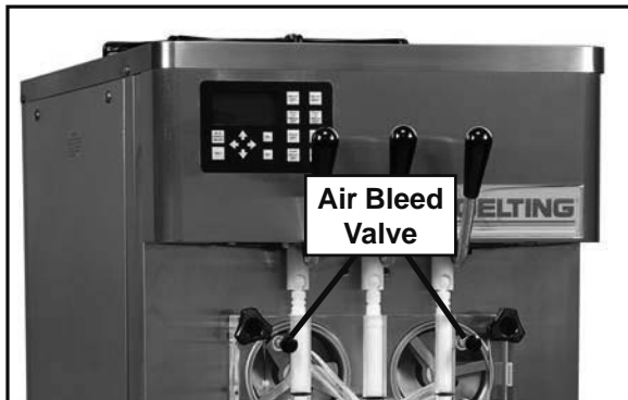
Figure 3-8 Air Bleed Valve
