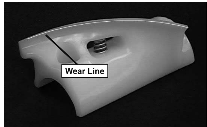
Figure 3-3 Auger Flight Wear
