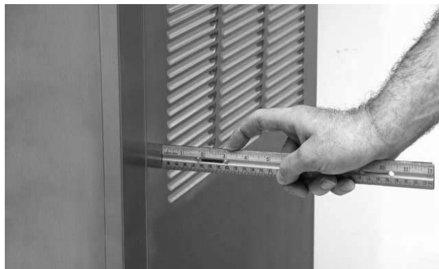
Figure 2-1 Space and Ventilation Requirements
