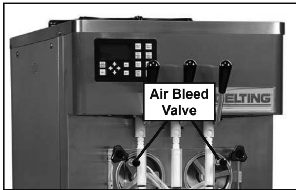
Figure 3-8 Air Bleed Valve
