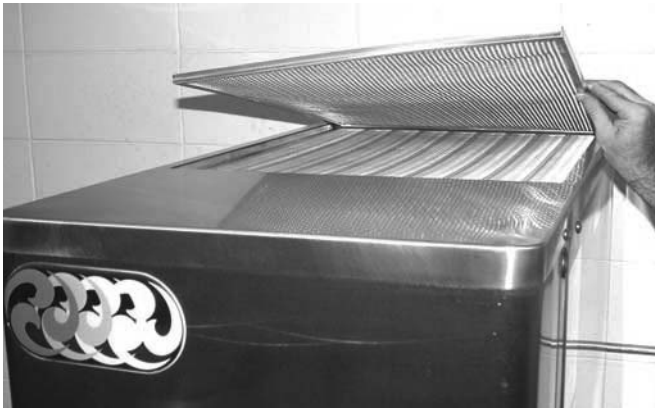
Figure 4-4 Removing Condenser Filter
