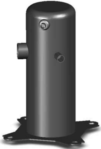
Figure 5-2 Scroll Type Compressor
