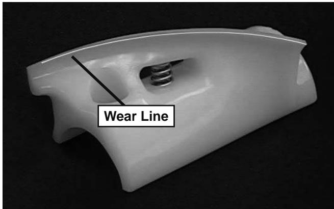
Figure 3-3 Auger Flight Wear
