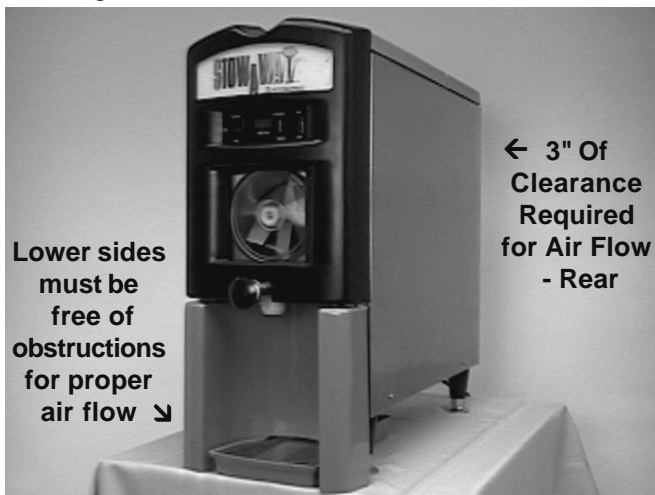
Figure 16. Clearance for Air Flow
