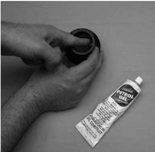
Figure 3-6 Lubricate Rear Seal
