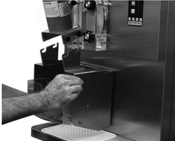
Figure 3-3 Removing Splash Shield Bracket
