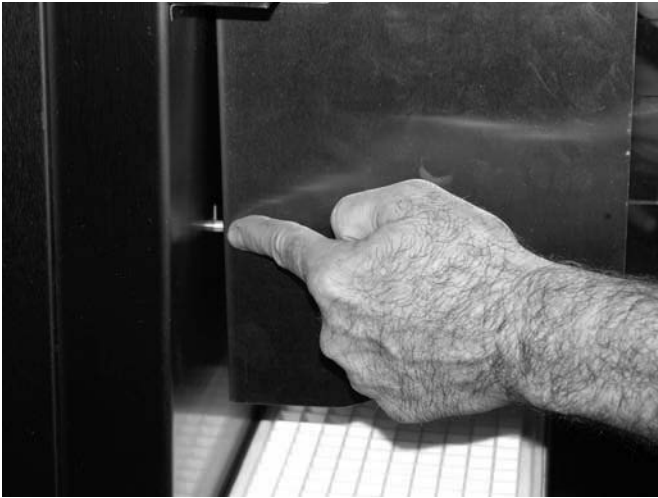
Figure 3-7 Blender Shroud Pin Alignment
