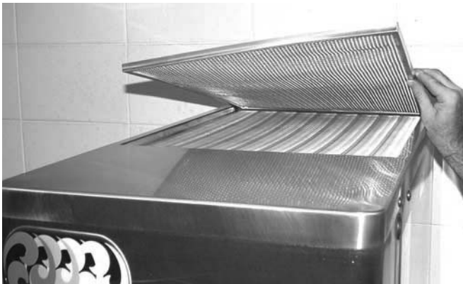
Figure 4-4 Removing Condenser Filter
