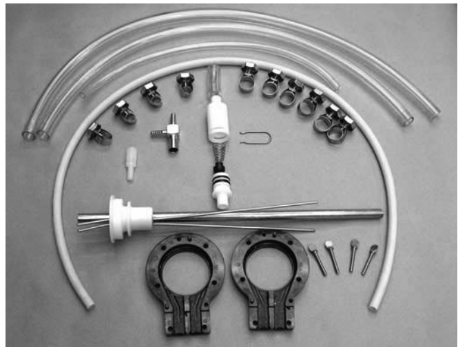
Figure 3-11 Mix Pump Removable Parts
