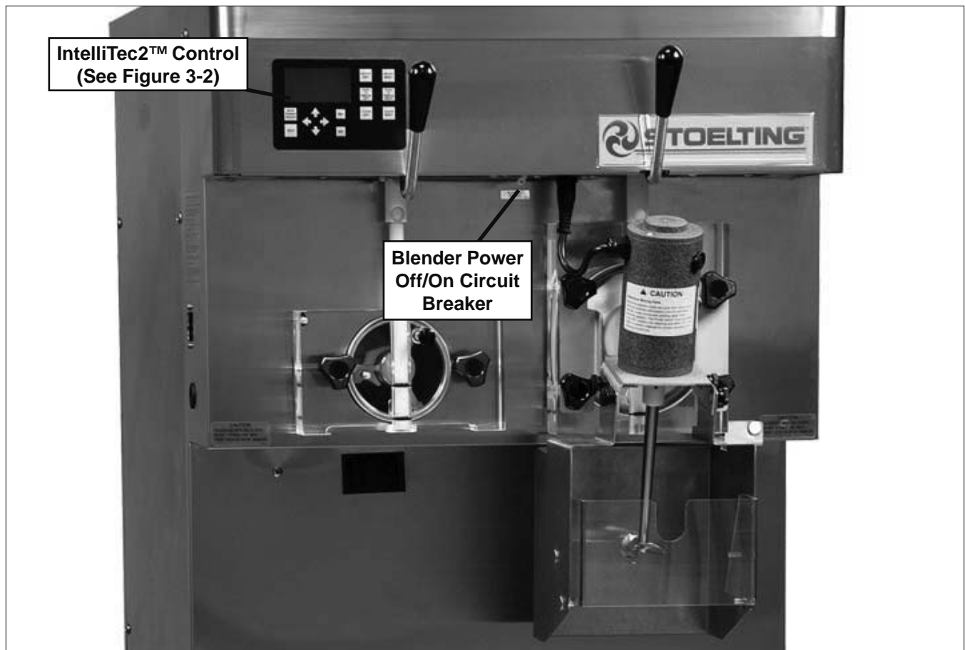
Figure 3-1 SU444 Freezer Controls
