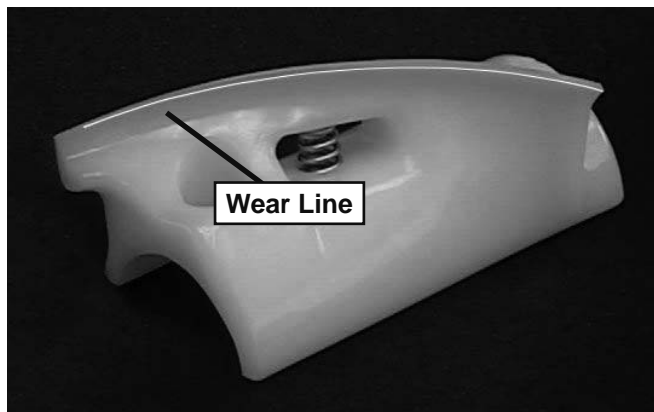
Figure 3-3 Auger Flight Wear
