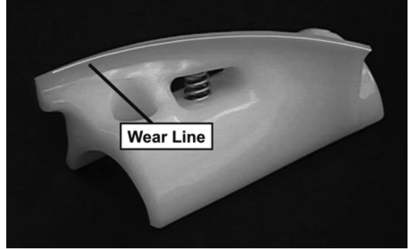
Auger Flight Wear
