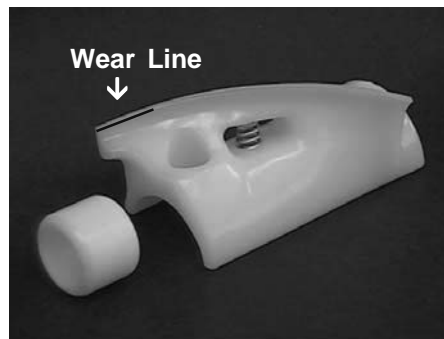
Figure 17. Auger Flight Wear & Front Auger Support Bushing Wear
