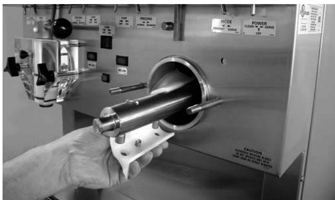
Figure 14. Auger Flight Removal
