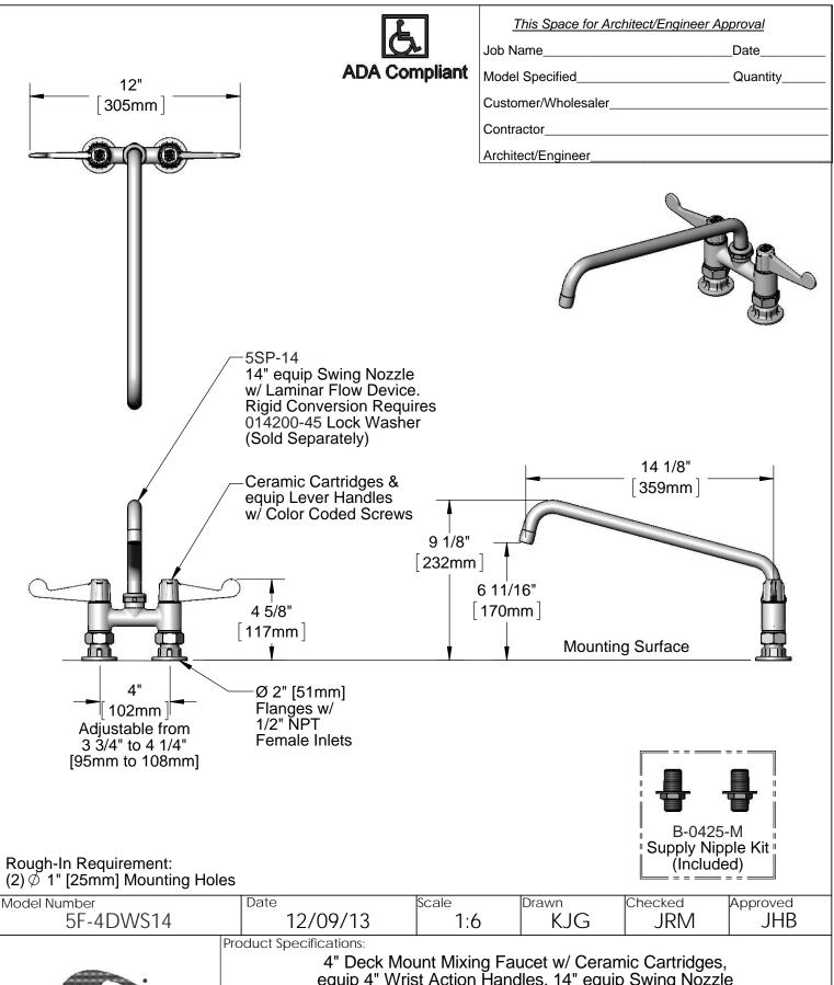
equip 4" Wrist Action Handles, 14" equip Swing Nozzle & 1/2" NPT Supply Nipple Kit
