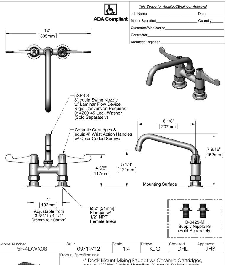
4" Deck Mount Mixing Faucet w/ Ceramic Cartridges, equip 4" Wrist Action Handles, 8" equip Swing Nozzle & 1/2" NPT Female Inlets
