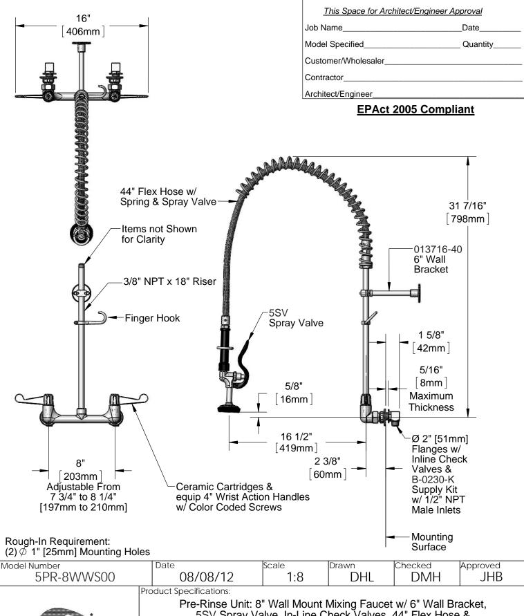
Pre-Rinse Unit: 8" Wall Mount Mixing Faucet w/ 6" Wall Bracket, 5SV Spray Valve, In-Line Check Valves, 44" Flex Hose & B-0230-K Supply Kit w/1/2" NPT Male Inlets
