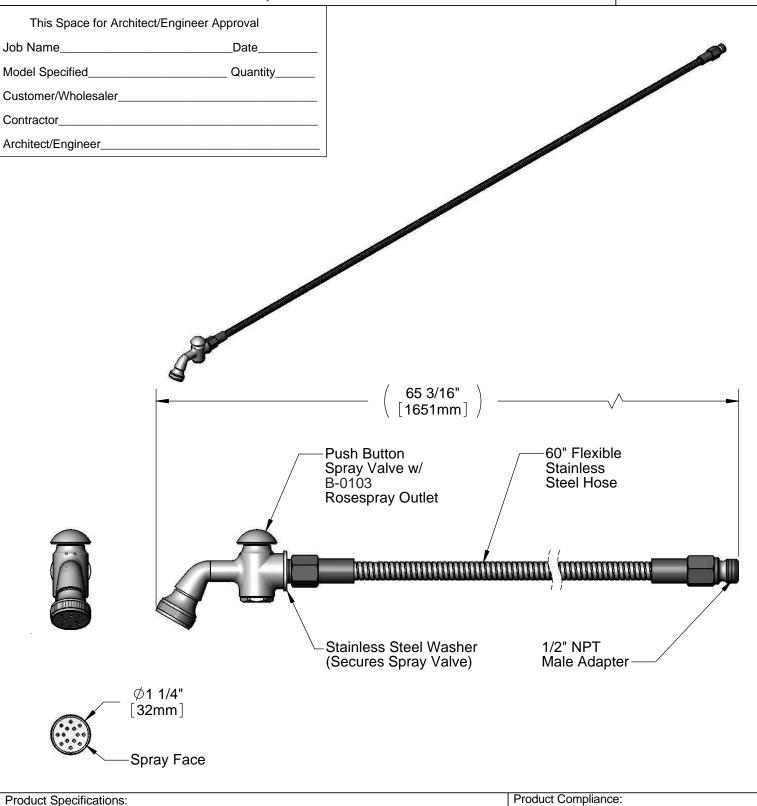
Spray Valve w/ Rosespray Outlet & 60" Flexible Stainless Steel Hose
