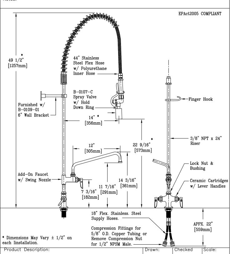
Easy Install Pre-Rinse Unit: Single Deck Mount Base Mixing Faucet, Flexible Supplies, Ceramic Cartridges, Add-On Faucet w/ 12" Swing Nozzle, 44" Flex Hose, Low Flow Spray Valve, Wall Bracket
