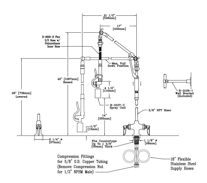
NOTE: For Backsplash Mounting, Riser Must Be Shortened To Maintain 14" [356mm] Clearance Between Spray Head And Fixture Flood Rim Level
