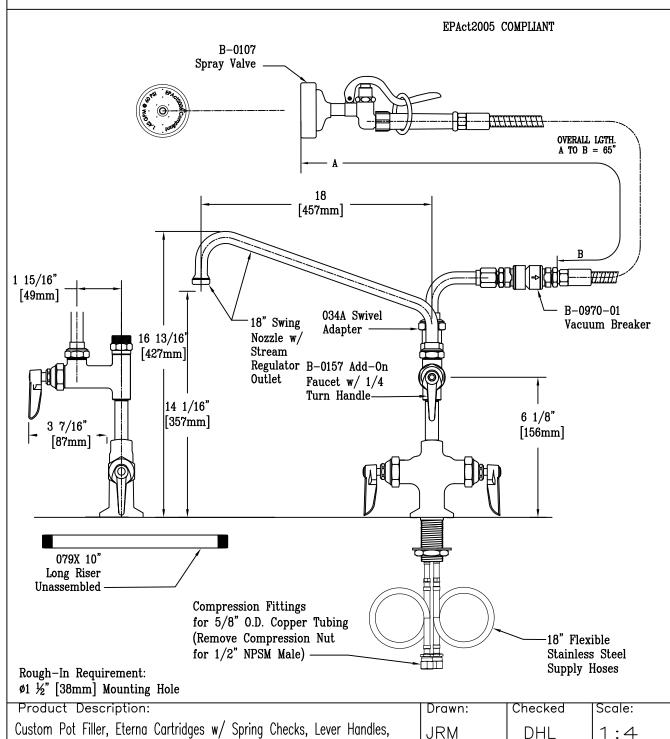
Custom Pot Filler, Eterna Cartridges w/ Spring Checks, Lever Handles, Vacuum Breaker, Add—On Faucet, 18" Swing Nozzle, Spray Valve, Optional Riser, 18" Flexible Stainless Steel Supply Hoses w/ 1/2" NPT Male Inlets
