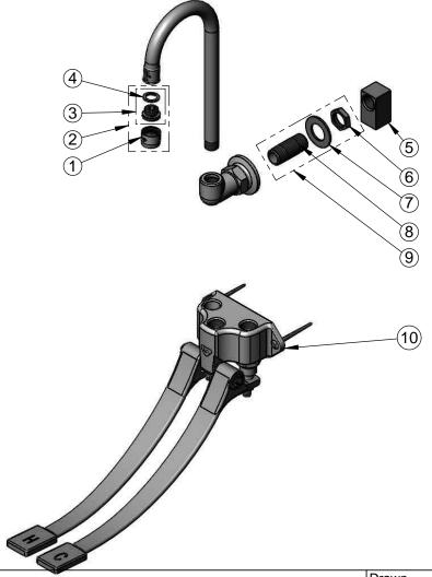
Product Specifications: Checked Approved Drawn Wall Mount Double Pedal Valve w/ Dummy Rigid Gooseneck & 2.2 GPM Aerator **KJG** DHL **JHB** Date: Scale: **NTS** 05/24/13
