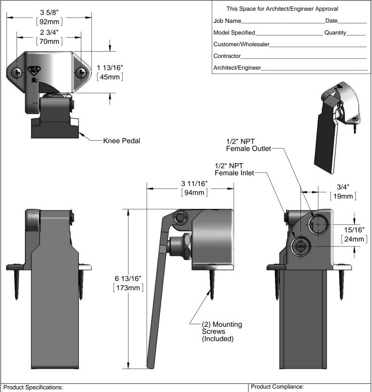
Knee Pedal Valve w/ 1/2" NPT Female Inlet & Outlet
