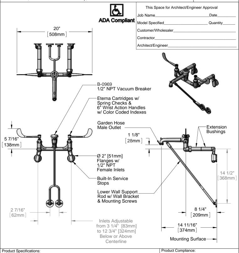
Adjustable Wall Mount Service Sink Faucet, Eterna Cartridges w/ Spring Checks, 6" Wrist Action Handles, Lower Support Rod, Garden Hose Male Outlet, Polished Chrome Finish, 1/2" NPT Vacuum Breaker & 1/2" NPT Extended Adjustable Inlets w/ Built-In Service Stops
