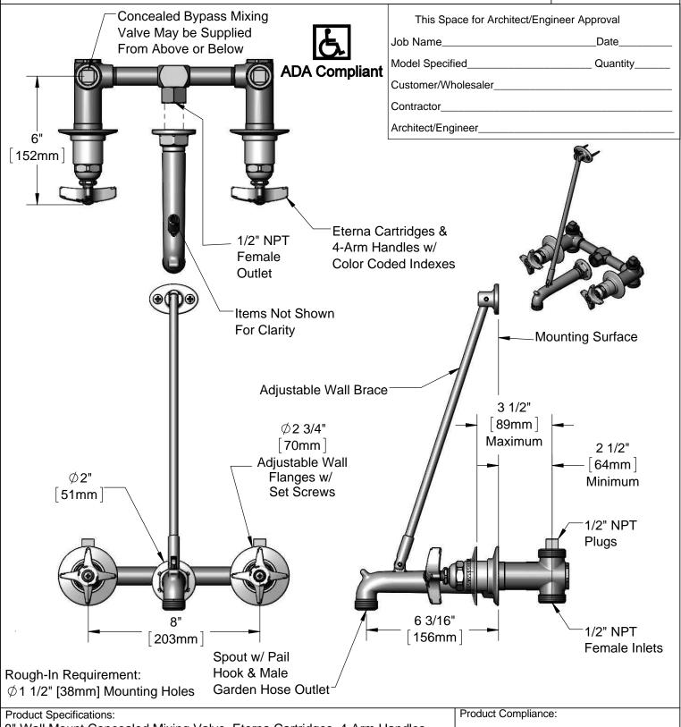
8" Wall Mount Concealed Mixing Valve, Eterna Cartridges, 4-Arm Handles, Spout w/ Pail Hook & Male Garden Hose Outlet, Upper Support Rod & 1/2" Female Inlets/Outlets
