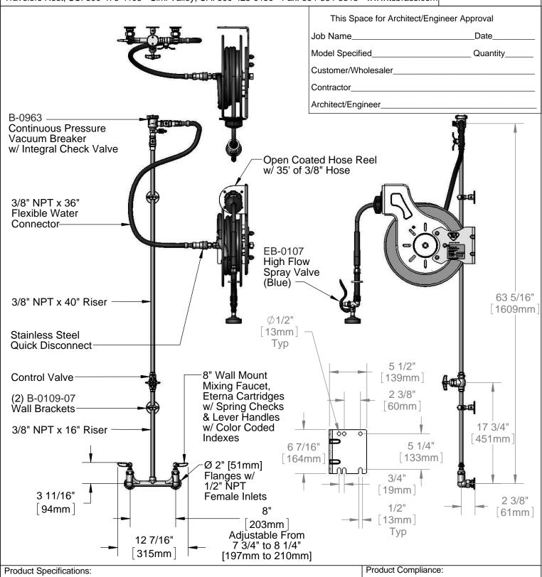
Open Coated Hose Reel w/ 35' of 3/8" Hose, High Flow Spray Valve (Blue), Vacuum Breaker, 3/8" NPT Flexible Water Connector, 8" Wall Mount Mixing Faucet & Control Valve
