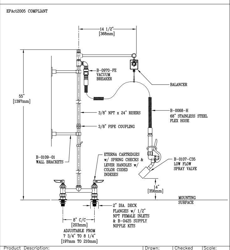
8" c/c DECK MOUNT PRE-RINSE UNIT w/ 1/2" NPT FEMALE INLETS, ETERNA CARTRIDGES SWIVEL RISER ASM, BALANCER ARM, WALL BRACKETS, 68" FLEX. ST. STEEL HOSE w/ LOW-FLOW SPRAY VALVE
