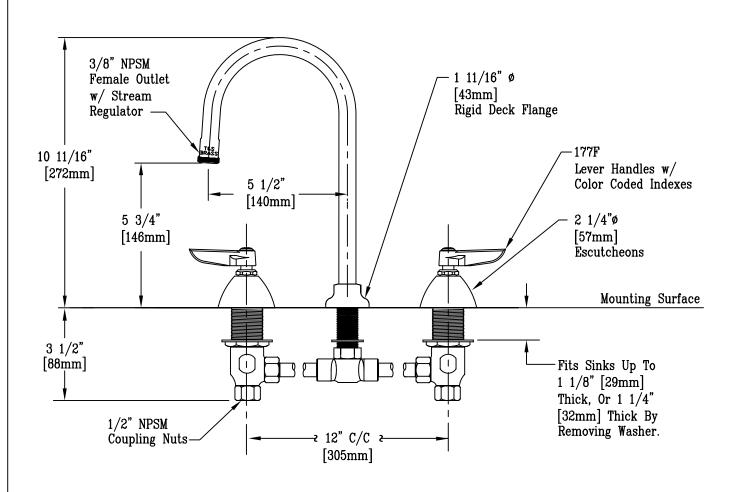
Note: Rough—in Required: \$\phi7/8\$ for Center Shank \$\phi1 1/4\$ for Hot/Cold Side Bodies
