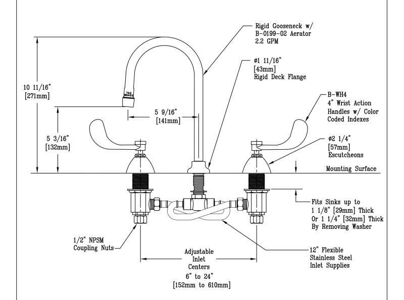
Note: Rough-in Required: Ø1" [25mm] for Center Shank Ø1 1/2" [38mm] Holes [1 1/4" [32mm] Minimum] for Hot/Cold Side Bodies
