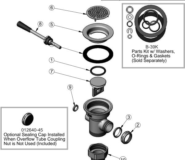
Approved **Product Specifications:** Drawn Checked Waste Drain Valve w/ Short Lever Handle, 3" Sink Opening, 2" NPT Male Outlet & 1 1/2" NPT Male Adapter **KJG GEF** Scale:
