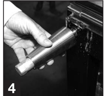
4 Thread leg into cabinet bottom frame rail.
