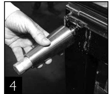
4 Thread leg into cabinet bottom frame rail.
