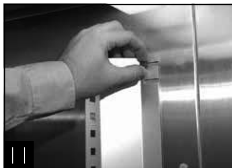
Pilaster installation two and three door models (middle of wall in rear of cabinet)
