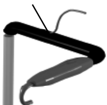
Accumulator, Capillary & Suction
