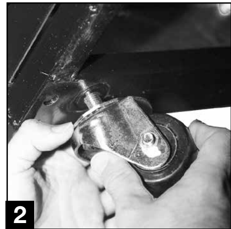
Thread castors into existing leg leveler holes.
