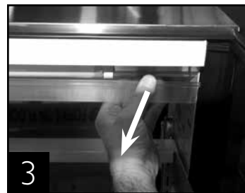
3 Squeeze lampshield and rotate out.
