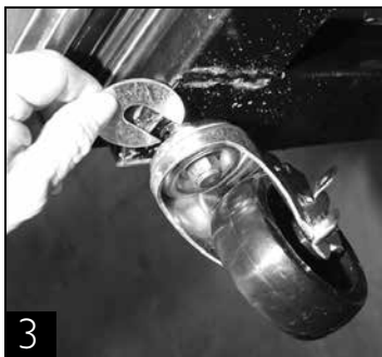
3 Use shims as necessary to level cabinet.
