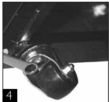
4 Tighten castor in position with castor wrench.
