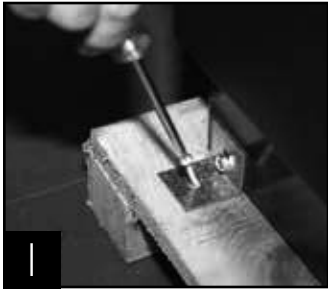
Removing bracket from skid.
