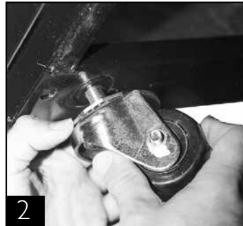
2 Thread castors into existing leg leveler holes.
