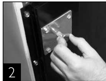
2 Reinstall leg levelers at bottom of cabinet.
