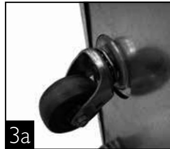
Installing castors (shims)
