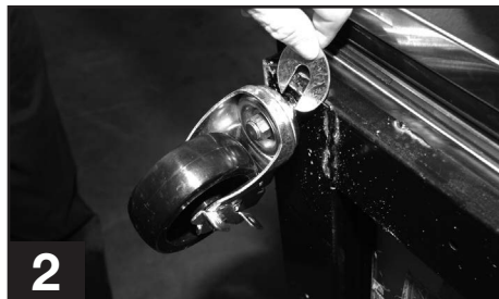
For leveling, insert the shim between the castor and frame rail.
