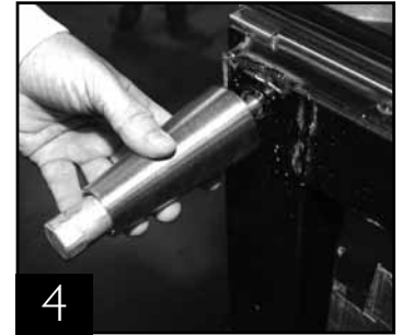
4 Thread leg into cabinet bottom frame rail.
