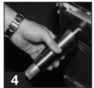
4 Thread leg into cabinet bottom frame rail.
