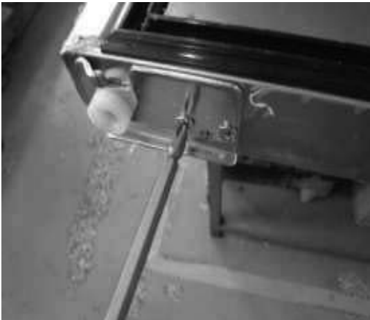
F. Disassemble stopper plate, then tight screws.
