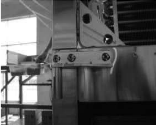
F. Disassemble stopper plate, then tight screws.
