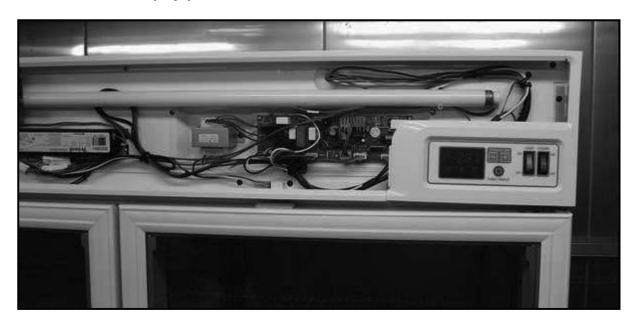
D. Replace parts as needed (Display board, Power switch, Lamp switch)
