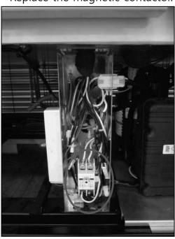
F. Disconnect connector to replace the SMPS
