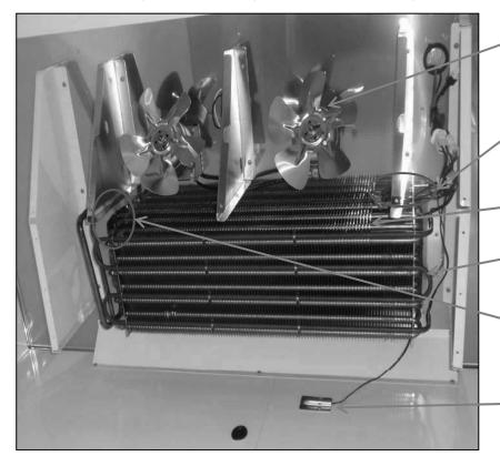
EVAPORATOR FAN MOTOR & BLADE
